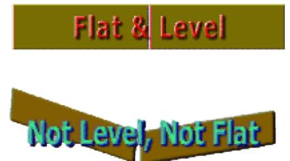
your working tile is not flat. Now, tap the tile slightly on the high side to bring it into flatness with all the adjoining tiles. They must all be flat, straight, level, and square.
